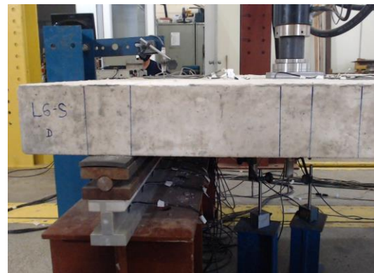
Figure 12 - Sketch of the instrumentation: a) side view showing the position of sensors; b) side picture of the test L6-S.
