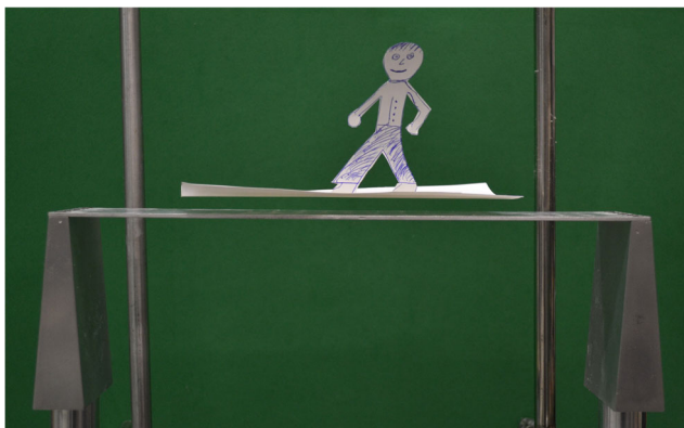
Fig. 16 Acoustic levitation of a slightly curved object by a levitation device consisting of two 25 kHz transducers attached to an aluminum plate of 300 mm in length. (Reprinted with permission from [151]; Copyright 2017, Acoustic Society of America)
