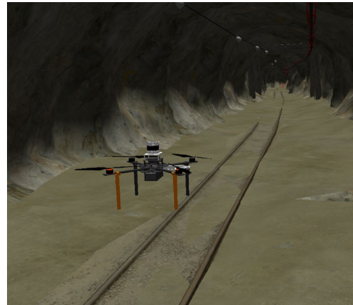
Fig. 11 Simulation visualization in Gazebo of Fly4Future T650 drone flying inside the underground tunnel
