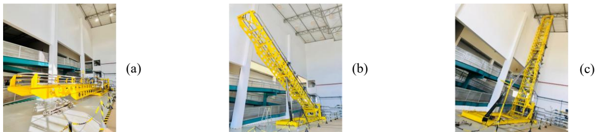
Figure 1. Inclinable multiphase flow platform of LEMI at (a) 0°, (b) 45° and (c) 90° inclinations, Ruiz-Diaz (2024).
