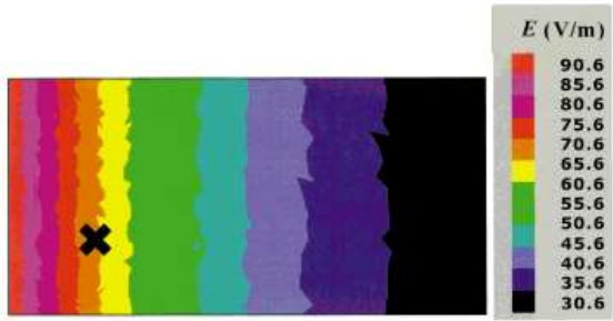
Figure 12 Visualization of the electric field in the resistor through color shades. The cross indicates the centroid of the element 1 of the mesh shown in Figure 9.
