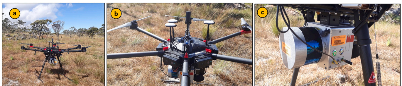
Fig. 3. GatorEye UAV-lidar (Gen 1) system. a) DJI M600 Pro hexacopter, with Phoenix Scout Ultra, hyperspectral, and visual sensors; b) three GNSS antennas for navigation, and one for sensor trajectory (positioned in the middle); c) Velodyne Ultra Puck lidar system.
