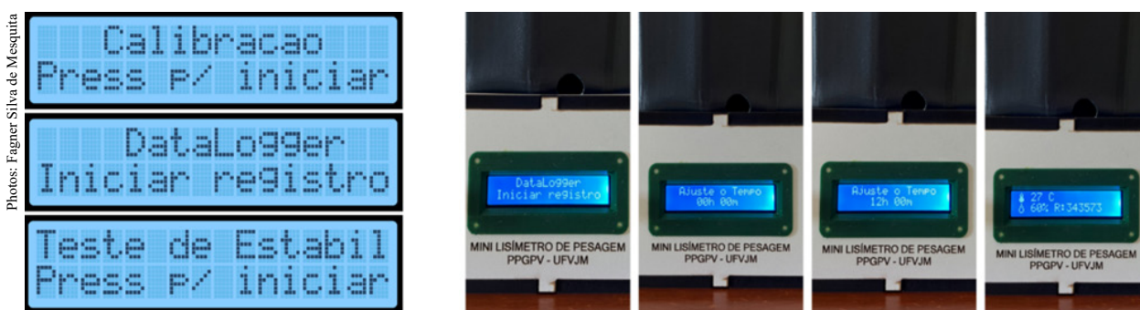
Figure 3. Interface and operation - navigation menu, functions, and variable readings.
