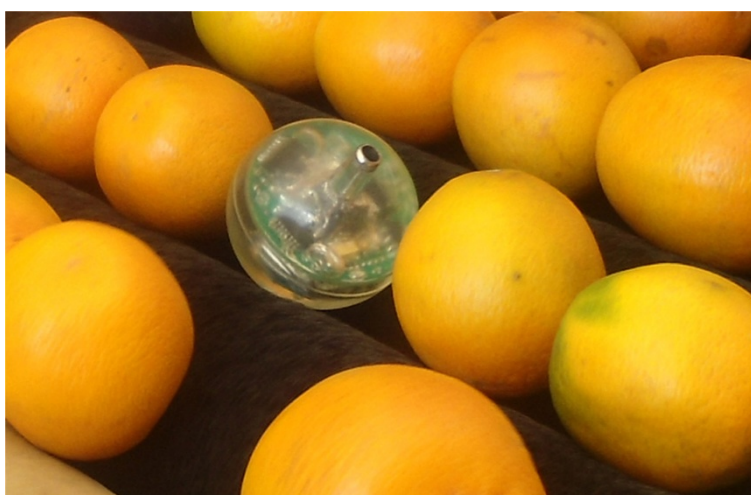
Figure 2 Wireless Instrumented Sphere (WIS).
