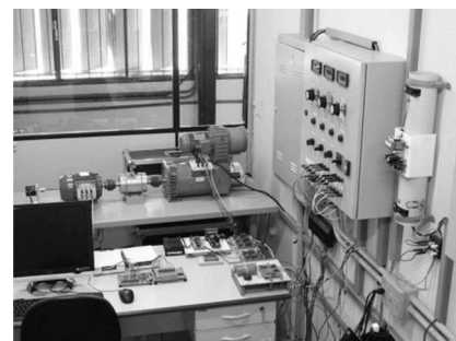
Fig. 5. Laboratory workbench with the 1-hp induction machine and data acquisition system.
