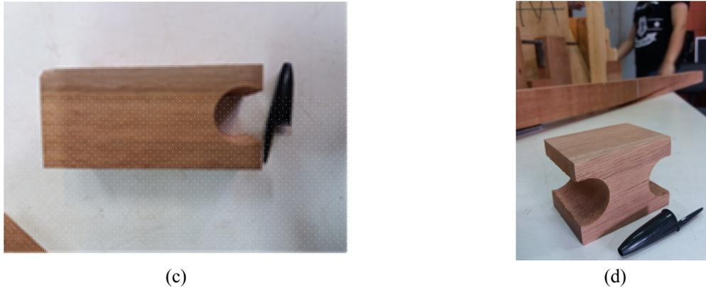
Fig. 1: (a) Dimension of wood specimens for compression, tension, shear strength and hardness and description of their extraction on timber (dimension in mm) (Morando et al. 2019); (b) toughness impact specimen; (c) splitting strength specimen; (d) normal tensile strength specimen.
