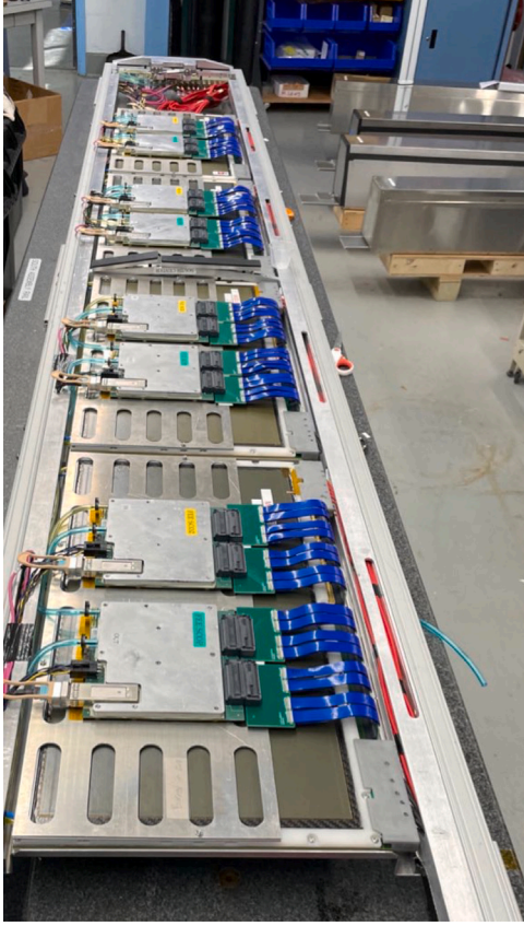
Fig. 9. Picture of the central TPOT sector, fully assembled, with four Micromegas modules, readout electronics, cooling plates and services.
