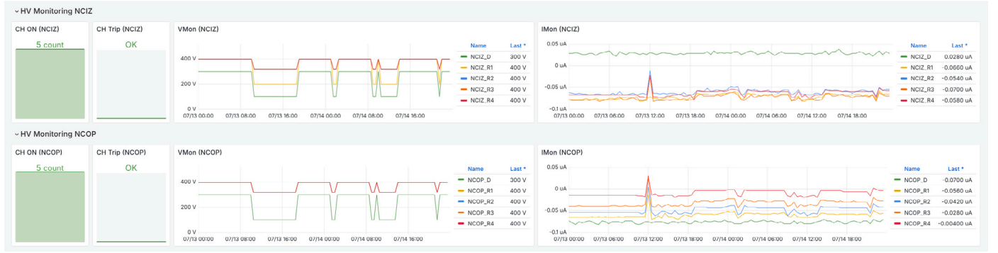
Fig. 21. Example of monitoring of the HV (left) and current (right) of two TPOT chambers over time. The low and high values on the HV panel correspond to TPOT being in either SAFE or ON state, respectively, depending on the presence of beam in sPHENIX.
