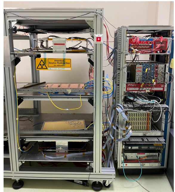
Fig. 24. Picture of the cosmic test bench used at Saclay for the characterization of the TPOT modules during production.
