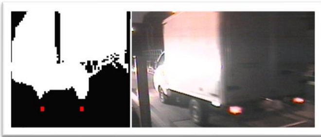
FIGURE 9. Example of a classification failure: a category 1 truck detected as a category 2 one.
