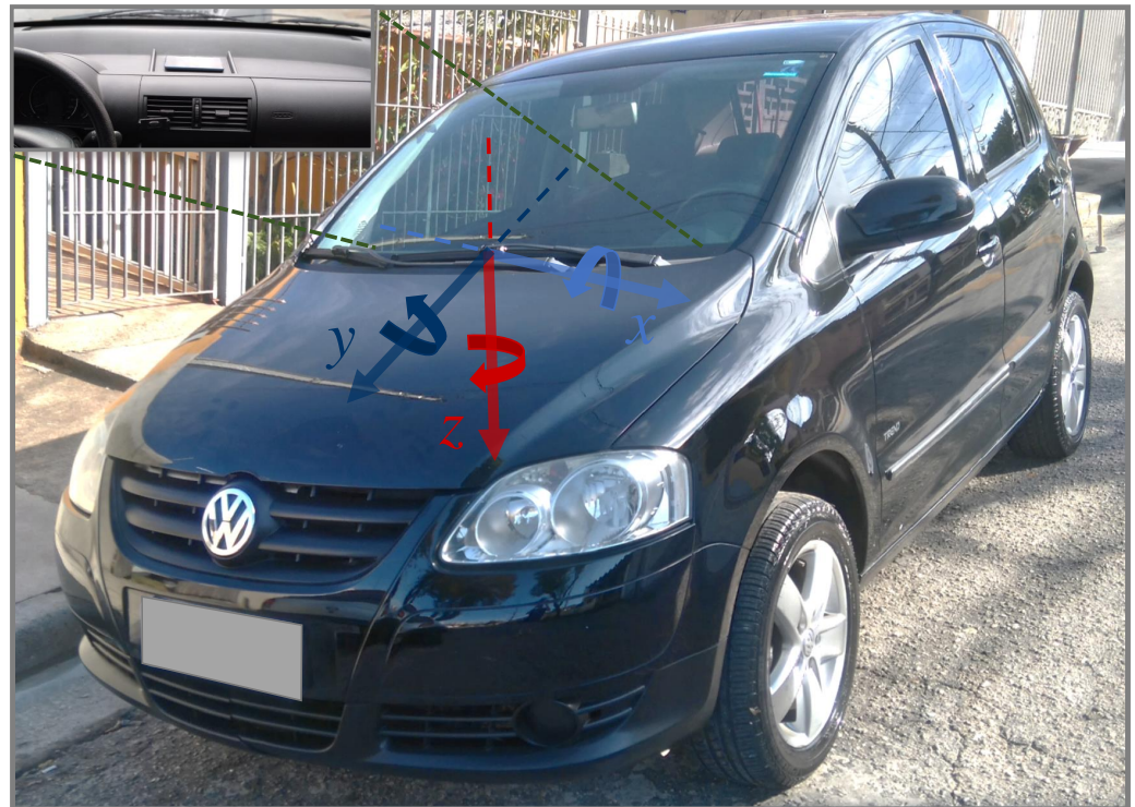
Figure 1. Smartphone installation location (in detail) and coordinate reference system x , y , and z . The x axis points to left and is perpendicular to the vehicle plane of symmetry. The y axis points forward and is parallel to the vehicle plane of symmetry. The z axis extends downwards. The pitch, roll, and yaw are the counterclockwise (right-handed) rotations about the x , y , and z axes, respectively.
