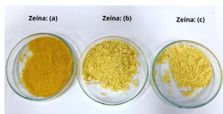
Figure 2: Zein extracted from: CGM(a); ground corn grains; (c) commercial from Aldrich
