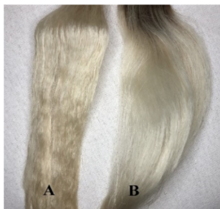
Figure 3. Appearance of bleached hair tress (T3): (A) after immersion in artificial seawater; (B) before immersion in artificial seawater.
