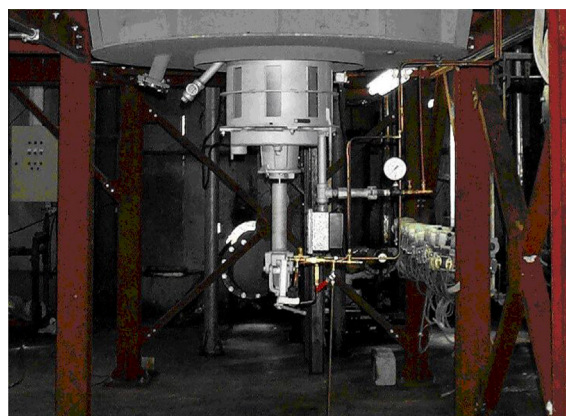
Fig. 1. Partial view of the vertical furnace used in the experiments.
