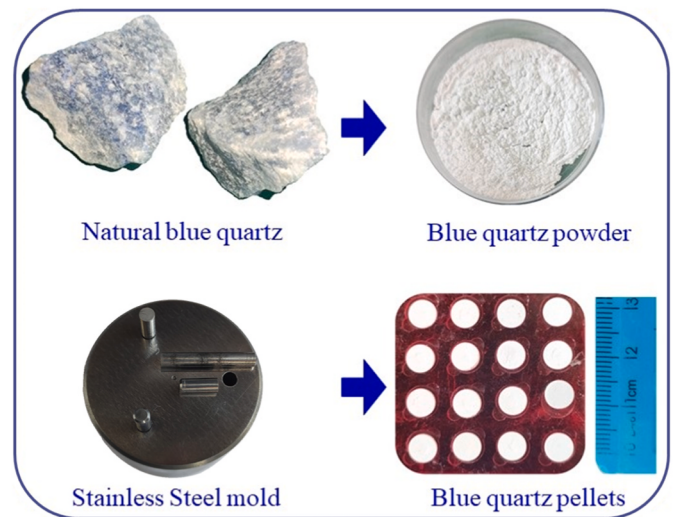
Fig. 1. (Top) Sample of the blue quartz crystal, as received and in powder form, was used to produce the pellets. (Bottom) Stainless steel mold used to press the sample and images of the blue quartz pellets sintered at high temperatures. (For interpretation of the references to color in this figure legend, the reader is referred to the Web version of this article.)
