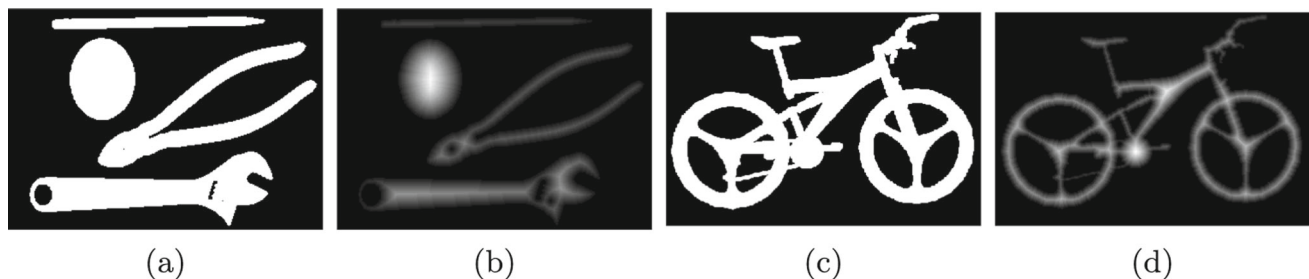
Fig. 5 Examples of DT computation by IFT with 8-connected adjacency. a & c Two given binary images X_1 and X_2 , respectively. b & d The corresponding DT values computed by IFT for all pixels in X_1 and X_2 , respectively. The DT error by IFT at pixel q is measured by \epsilon(q) = |\text{edt}(X, q) - \sqrt{\Psi_{\text{Euc}}(\pi^*(p, q))}| , with \pi^*(p, q) the path com-
