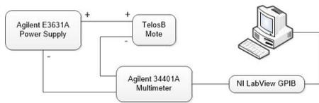
Fig. 2. Power consumption measurement setup.
