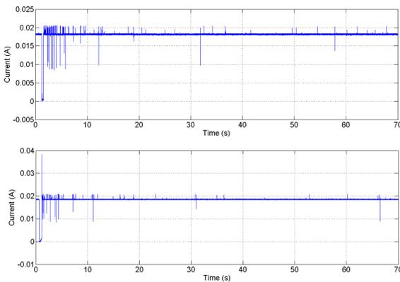
Fig. 3. CTP: current measurement on root (top) and leaf (bottom) nodes.
