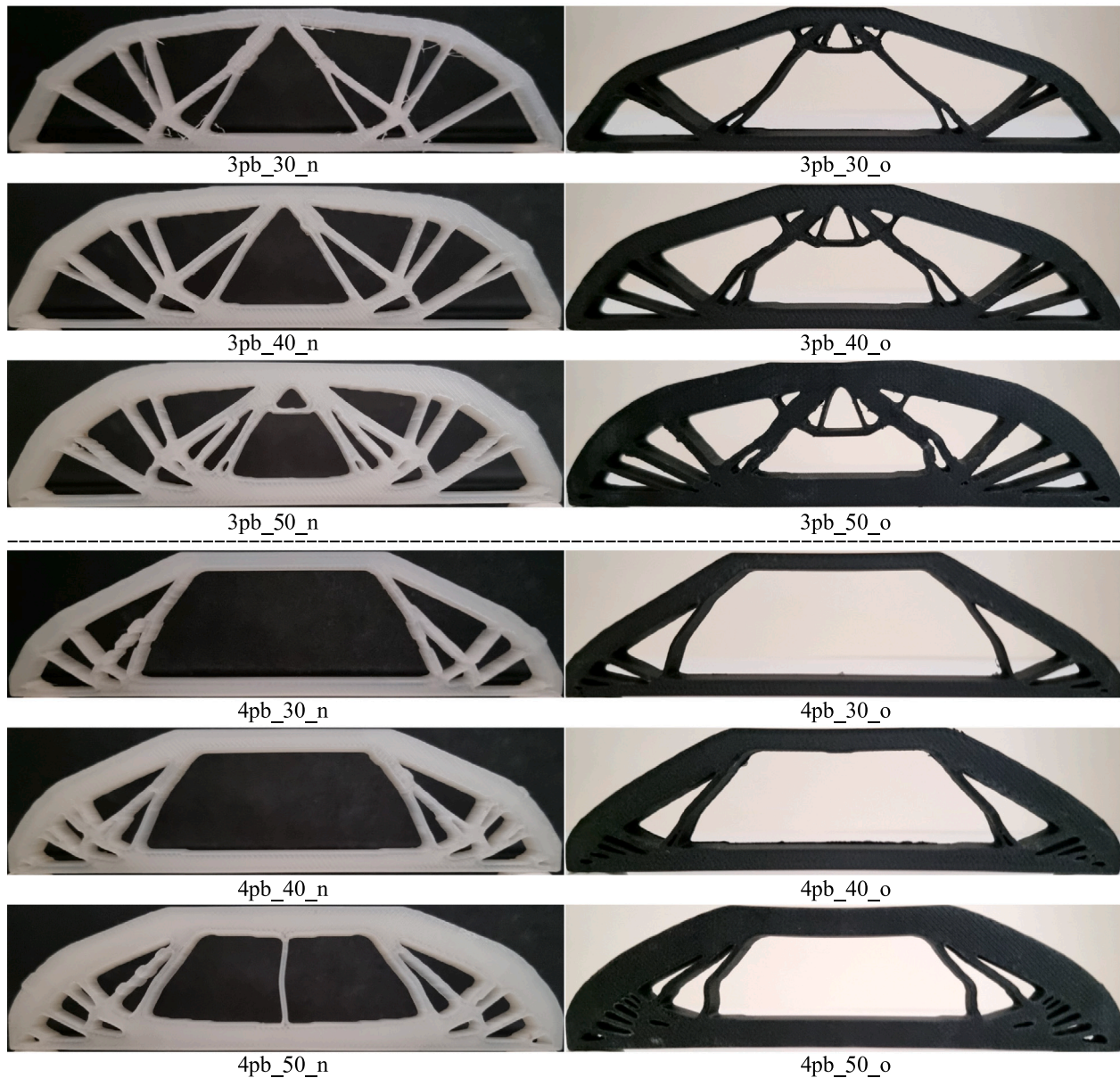
Fig. 11. Deformed shapes for all 3D printed parts after unloading.
