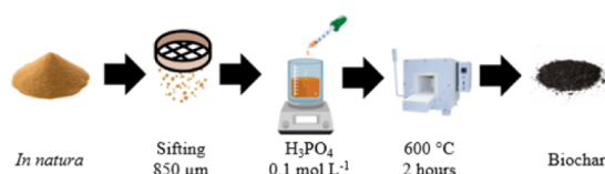
Figure 1. Schematic representation of the biochar synthesis process from Lagenaria siceraria waste.
