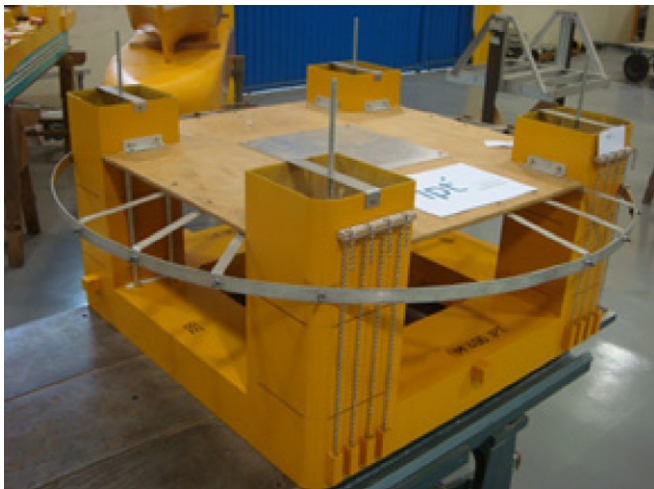
Fig. 6. Picture of the semi-submersible model scaled in 1:100.
