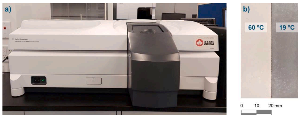
Fig. 1. a) Cary 5000 UV-VIS-NIR; b) TC+P25 samples above and below TT.
