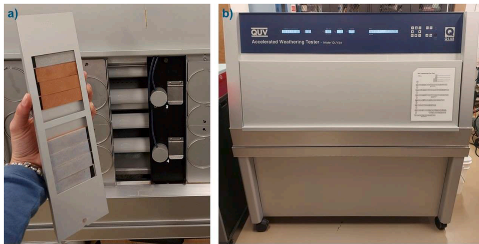
Fig. 2. Weathering apparatus: a) sample holder and UV lamps; b) QUV machine.
