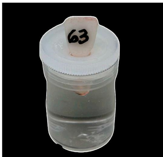
**Figure 1.** Experimental model showing a tooth specimen placed in an acrylic pot containing 10 mL of phosphate-buffered saline (PBS), with only the root portion immersed in the solution.
