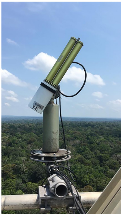
Figure 1: Cimel sun photometer from the AERONET network at the Amazon Tall Tower Observatory (ATTO) site.
