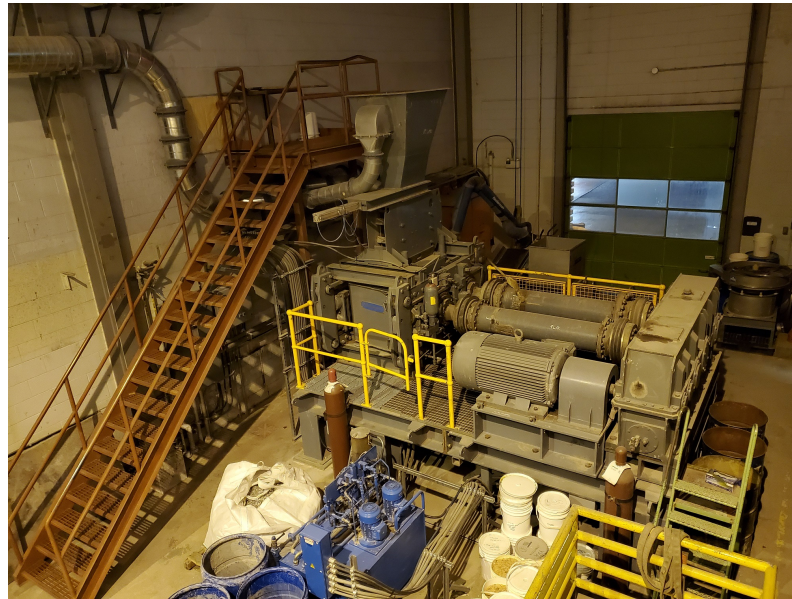
Figure 1. Köppern pilot-scale HPGR at UBC used to run the tests.
