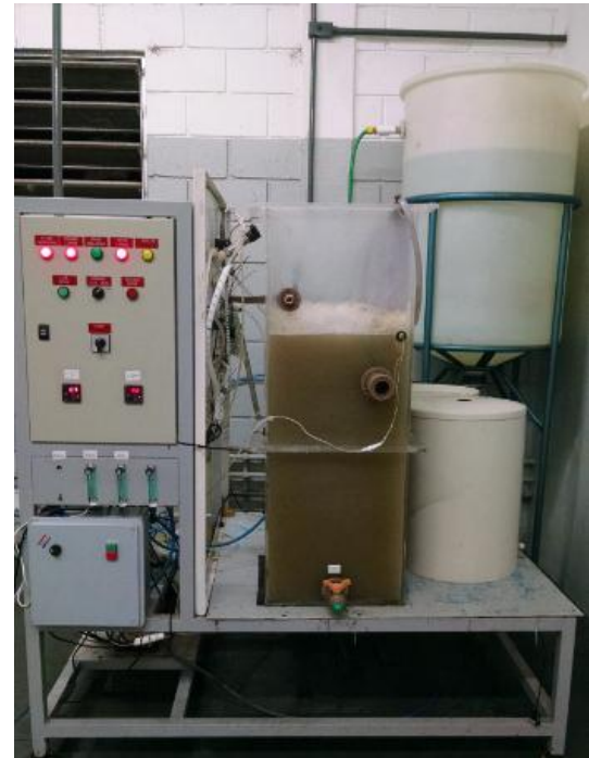
Figure SM_1. Simplified scheme (a) and photograph (b) of the MBR system used in this study.
