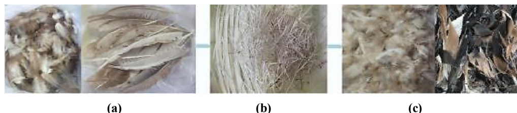
Figure 1: Samples Preparation: Down Feather and Feathers Raw Respectively (a); Rachis (b) and Down Feather and Feather Fibers Respectively (c) (ASTM D 4524/12 and NF EM 1883/98)
