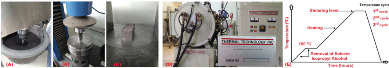
Fig. 2. (A) Conventional stirrer with a capacity of 3 kg of mixtures. (B) Compaction of specimens. (C) Rectangular samples of green compacts for the LPS process. (D) Vacuum sintering furnace; (E) sintering thermal cycle. (For interpretation of the references to colour in this figure legend, the reader is referred to the web version of this article.)
