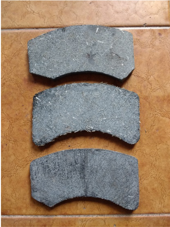
Fig. 2 – General appearance of the friction elements prepared.
