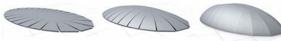
Figure 25. “Pneumatic Forming of Hardened Concrete (PFHC)” construction process. Adapted from [30].
