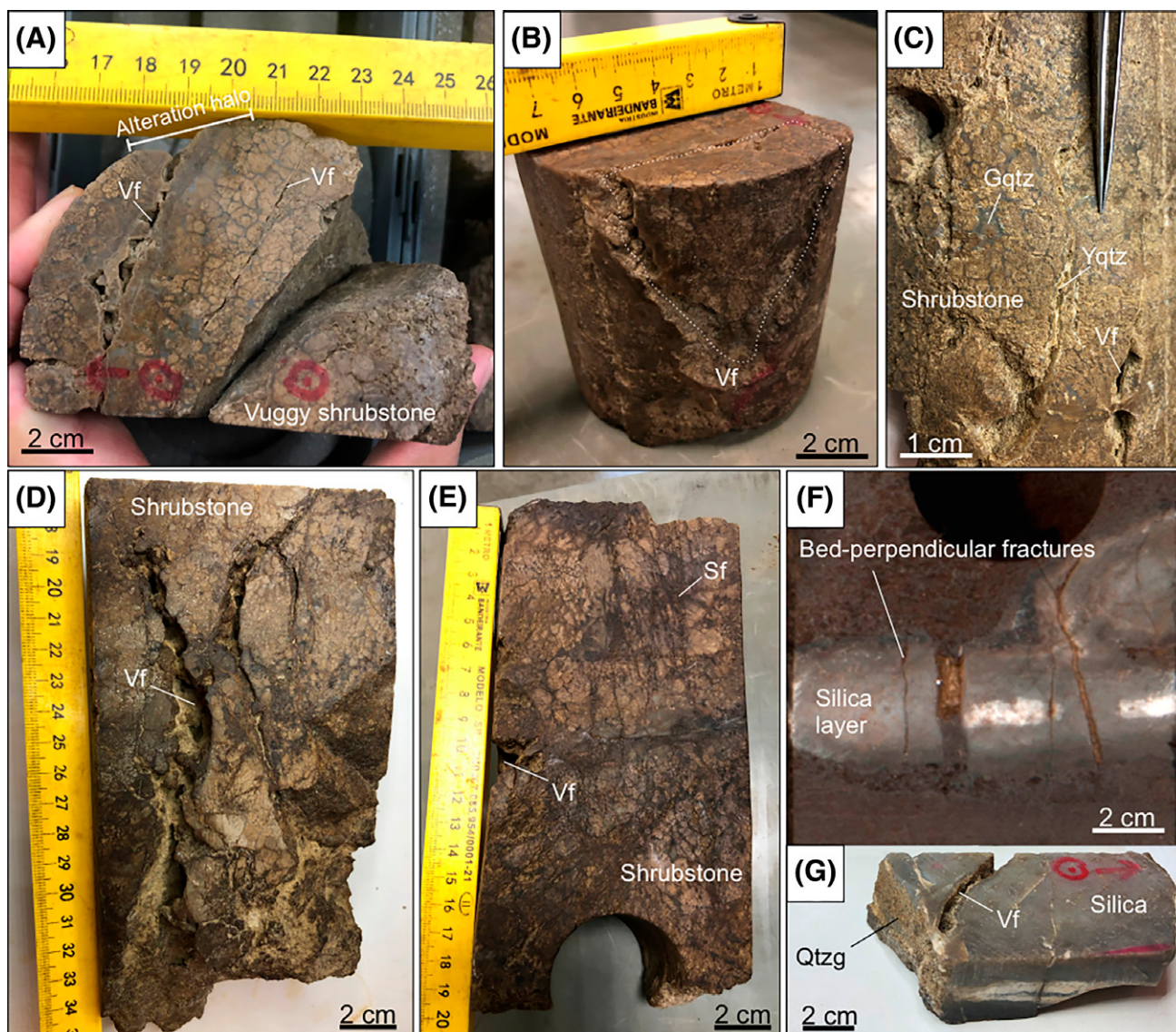
Figure 3. Fracture and dissolution features observed in the core from well A. (A) Vuggy fracture (Vf) cutting the shrubstone host rock with alteration halo. Most primary pores of the host rock are filled with grayish quartz. Host rock is commonly observed with vuggy aspect. (B) The Vf crossing the core. Vugs are coated with up to 1-mm-sized euhehedral quartz crystals. (C) The vuggy fractures filled with yellowish quartz (Yqtz) and shrubstone host rock cemented with grayish quartz (Gqtz). Sparse vugs or geodes filled by quartz crystals are observed in the host rock. (D) The vuggy fractures with centimeter-sized aperture coated by euhehedral quartz. (E) Narrow small displacement fault (Sf) swarm, with cataclastic fill. (F) Silica layer bearing bed-perpendicular opening-mode fractures. (G) Silicified spherulitstone host rock and open Vf with euhehedral quartz. This fracture is associated with centimeter-sized quartz geodes (Qtzg).
