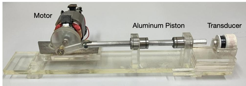
**Figure 7.** System built for the mechanical stimulation of the transducers.
