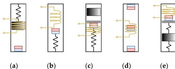
**Figure 3.** Linear EM energy harvesting architectures: (a) spring-mass with moving coil; (b) spring-mass with moving magnet; (c) free impact mass frequency-up converter; (d) magnetic levitation; and (e) double spring-mass with moving magnet.
