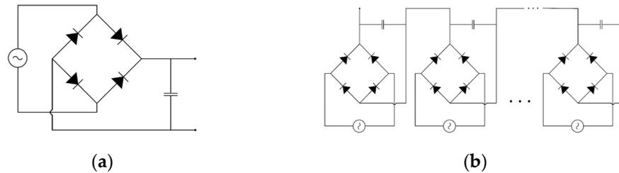
**Figure 6.** (a) Schematic of the full-wave rectifier circuit; (b) in-series association of full-wave rectifier circuits.
