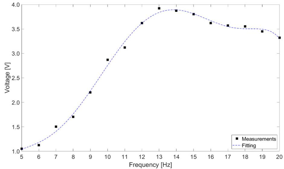
**Figure 9.** Voltage measurements at the output capacitor of the rectifier circuit connected to the energy harvester for input signals with frequencies from 5 to 20 Hz.
