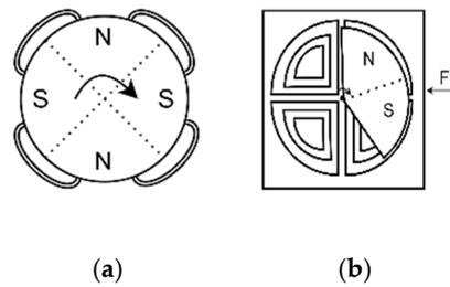
**Figure 4.** Non-resonant EM energy harvesters: (a) rotational, steady torque conversion (b) hybrid, converts linear to rotational movement.
