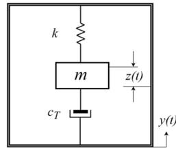
Figure 2. Linear electromagnetic energy harvester model.
