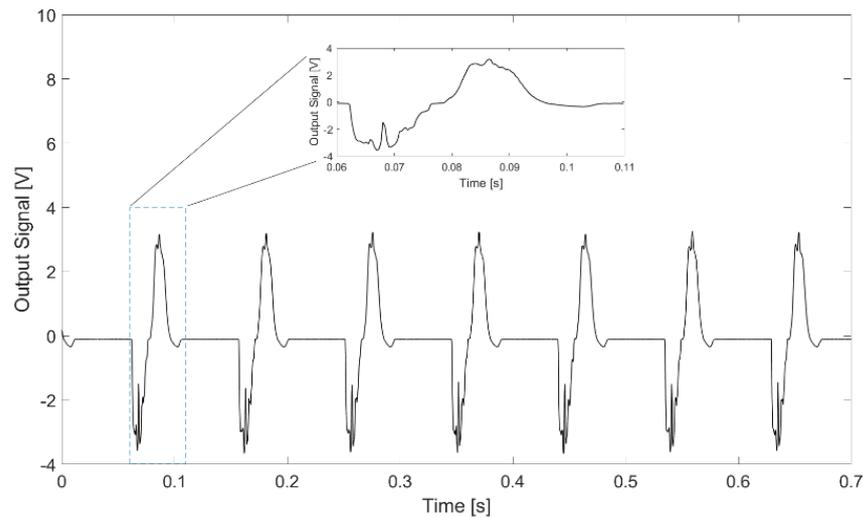
**Figure 8.** Signal generated by the energy harvester when excited with a harmonic signal of 10 Hz frequency, with a selected segment of the signal.
