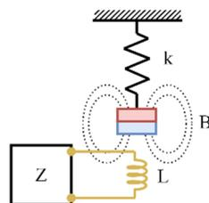
**Figure 1.** General linear electromagnetic energy harvester scheme.
