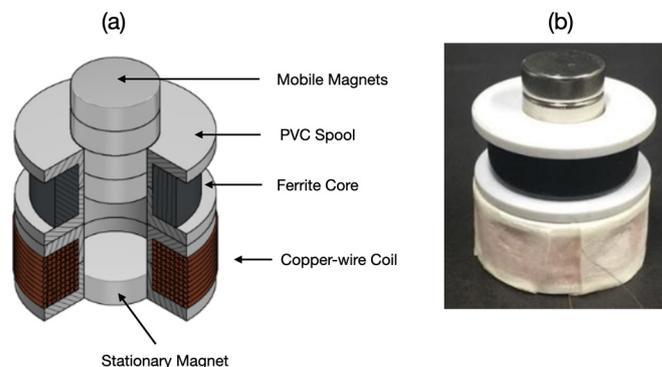
**Figure 5.** (a) Schematic of the developed energy harvester: coil with an air core, ferrite, four levitating magnets, and one fixed magnet; (b) final assembly.
