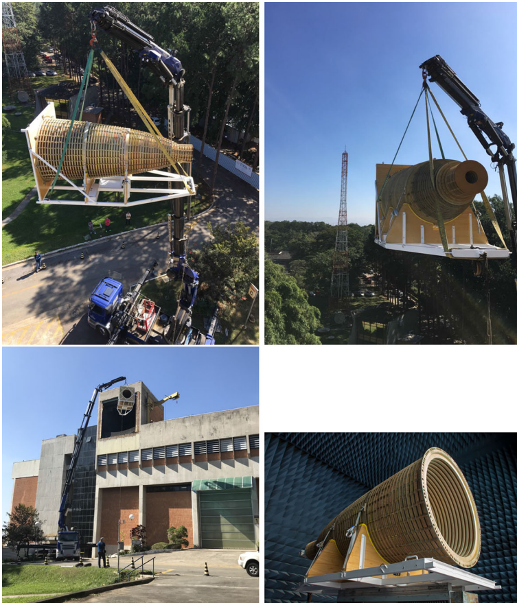
Fig. 8 Top left, top right and bottom left: Horn being suspended, with its cart, to the opening of the anechoic chamber of LIT test facility. Bottom right: The horn mounted inside the anechoic chamber.
