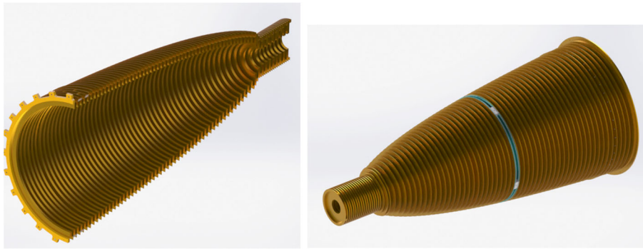
Fig. 3 Left: horn longitudinal cut through ring diameters. Right: Opposite view, with a suspension point in a machined ring in the middle of the horn (green ring)
