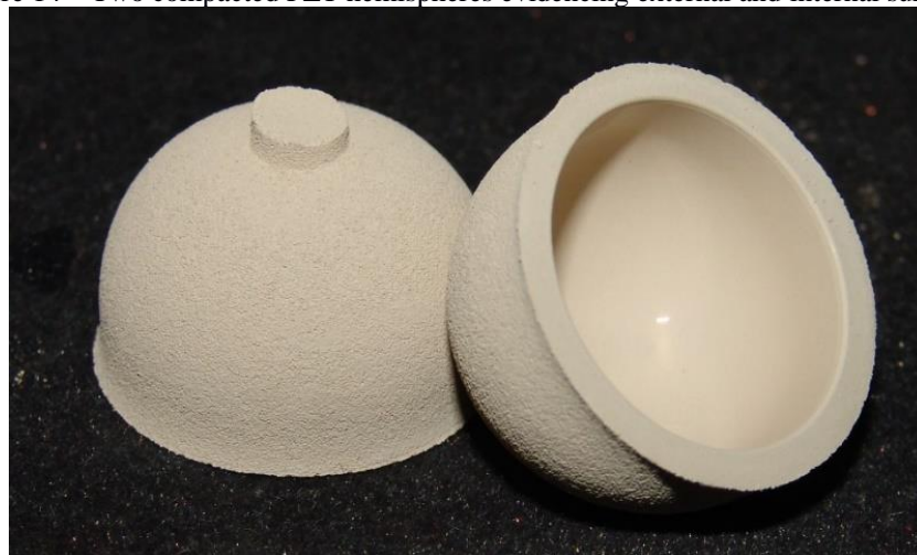
Figure 14 – Two compacted PZT hemispheres evidencing external and internal surfaces.
