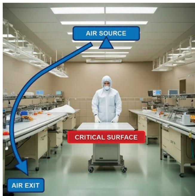
**FIGURE 7** - Non-laminar air flow.
