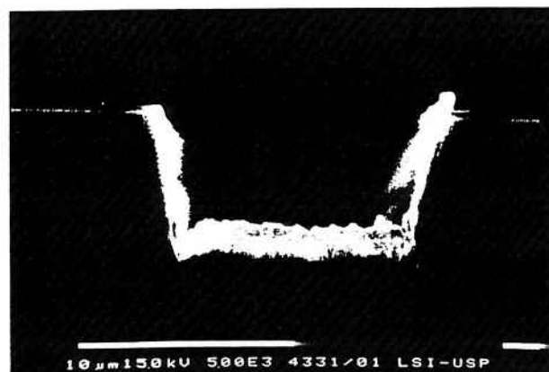
Fig. 2. Profile of a 10 \mu\text{m} wide trench, with the following etch process: 90% \text{CBrF}_3 flow, 10% \text{SF}_6 flow, 100 W power, stainless steel electrode, etch time 30 min. 100 nm of PECVD oxide was deposited to enhance the contrast.
