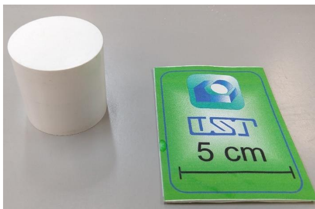
Figure 1 – Partially sintered core plug. It was the only sample that used an aqueous solution of polyvinyl alcohol instead of polyvinyl butyral as the binder.
