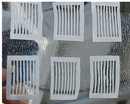
Figure 4. The result of the electret thermoforming process using the PTFE grid.
