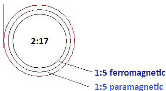
Fig. 9. The two shell layers of \text{Sm}(\text{Co,Cu})_5 phase surrounding the 2:17 main ferromagnetic phase. The first layer, cobalt-rich and ferromagnetic, results in exchange coupling. The second layer, copper-rich and paramagnetic, promotes magnetic decoupling between the 2:17 nanocells. Schematic.
