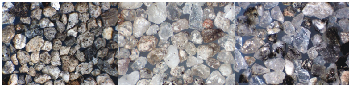
(a) <2.2 \text{ g/cm}^3 (b) 2.6 < d < 2.64 \text{ g/cm}^3 (c) d > 2.64 \text{ g/cm}^3 Figure 2: Stereoscope images of heavy liquid separation products (fraction -1.2 + 0.60 \text{ mm} ).
