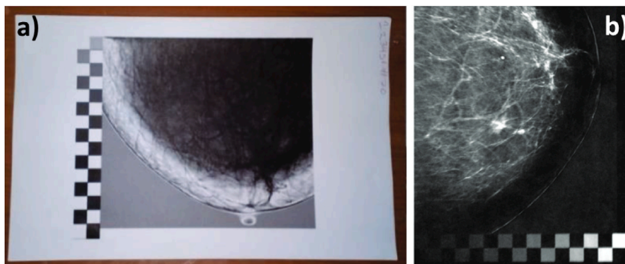
Fig. 10. Physical breast phantom created from bond paper with desktop inkjet printer and contrast medium: a) top view of a paper physical breast model and b) the corresponding mammography image. Reproduced from Manzano-Hernández et al., AIP Conference Proceedings 2090, 030004, (2019); used in accordance with the Creative Commons Attribution (CC BY) license ( https://creativecommons.org/licenses/by/4.0/ ).
