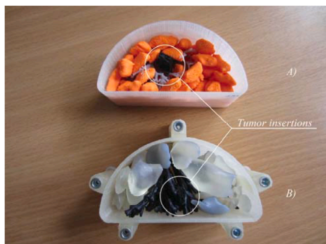
Fig. 6. Modular breast phantoms 3D printed at the Medical University of Varna (Bulgaria). The envelopes and the simulated tumors are manufactured with FDM technology and adipose compartments are developed via SLA technology. The duct tree is developed by means of FDM in a) and SLA in b). © 2019 IEEE. Reprinted, with permission, from Dukov et al. (2019b) An approach for printing tissue-mimicking abnormalities dedicated to applications in breast imaging. In 2019 IEEE XXVIII International Scientific Conference Electronics (ET) (pp. 1–4), IEEE.
