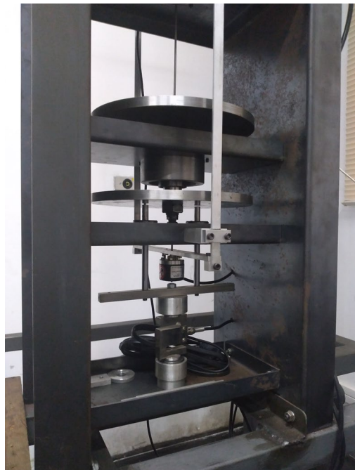
Fig. 7 Main disk and friction pins in test bench
