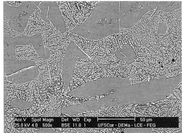
Figure 6. Steel modified with 0.5% niobium: annealed and aged for one hour at 850 °C. Laves phase appears as needles associated with sigma phase. BSE after Behara etching.
