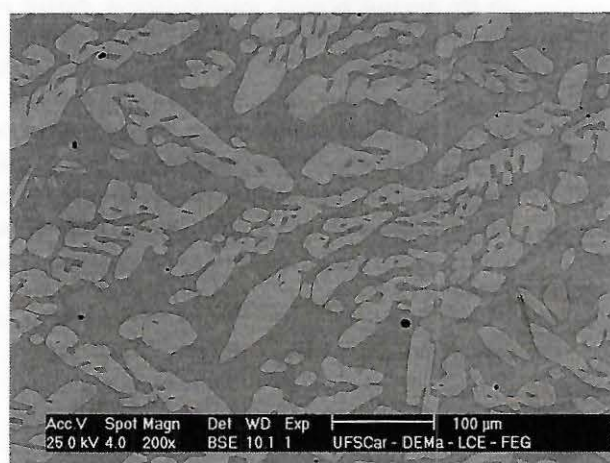
Figure 1. Steel without niobium: annealed sample shows elongated austenite grains in ferritic matrix. BSE after Behara etching.
