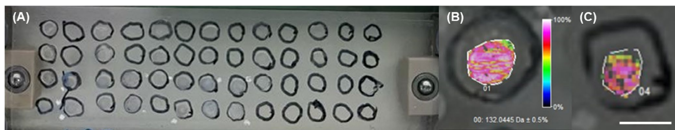
FIGURE 7 (A) Films positioned on ITO slide glass sample plates (A); MALDI-TOF imaging showing the distribution of ALA ( m/z=132.030 ) in the films (B) without ozone and (C) after ozone decontamination. The white scale bar at the bottom right represents 2 mm.
