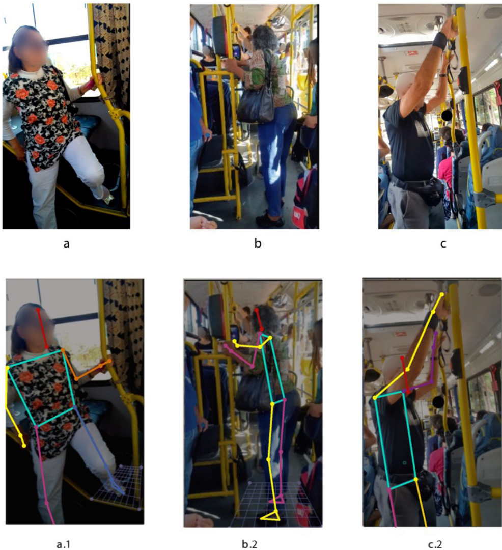
Figure 12. Demanding postures at the travelling stage: images a-c are part of the photographic evidence from observations with 3 participants during the travelling stage. Images a.1-c.3 depicts the images treatment using software Kinovea for analysis and postural assessment.
