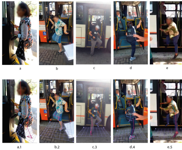
Figure 14. Demanding postures at the alighting stage: images a-e are part of the photographic evidence from observations with 5 participants during the alighting stage. Images a.1-e.5 depicts the images treatment using software Kinovea for analysis and postural assessment.
