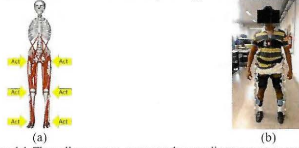
Figure 1. (a) Interaction model. The yellow arrows represent the coordinate actuators and the red lines represent the muscles. (b) User wearing the ExoTAO.
