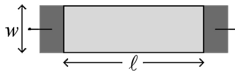
Fig. 1. Schematic of the implantation targets on which the conducting polymer samples are formed.
