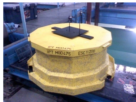
Fig. 4 Picture of the model made with polyvinyl chloride (PVC)
