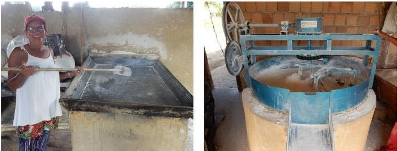
Fig. 6 Manual (left) and electric oven (right) used for roasting cassava flour
