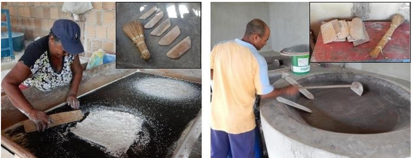
Fig. 7 Manual ovens used for production of cassava flour and beiju (on the left), with artisanal tools displayed in the upper right-hand corner of each photo
